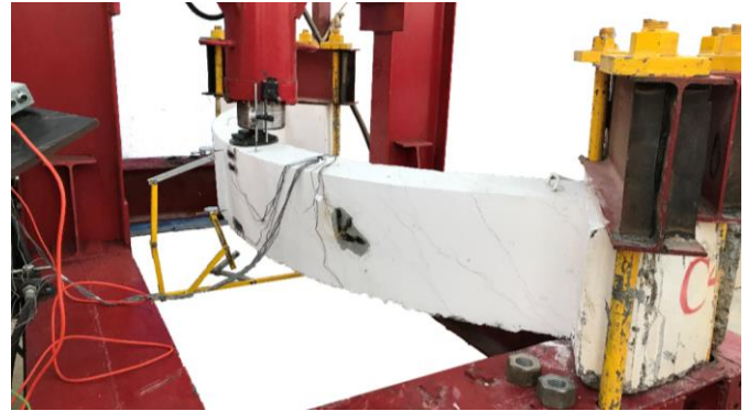
Fig. 4 Testing rig with beam C4.
