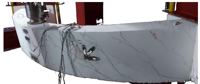
Fig. 11 Specimen C5 failure.
