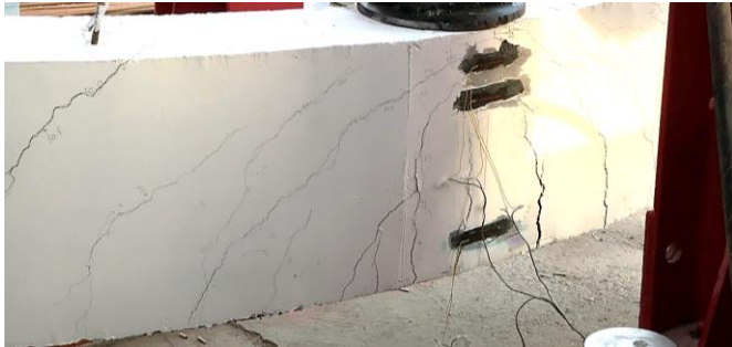
Fig. 7 Specimen C1 failure.
