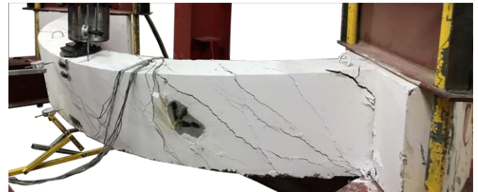
Fig. 10 Specimen C4 failure.
